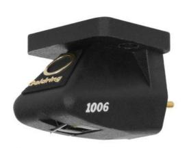
This hand-built cartridge features an elliptical stylus; its shape enables it to more accurately trace the highest frequency record grooves giving it the advantage over ordinary spherical types. The lightweight shank also gives the stylus a lower tip mass than cheaper metal bonded types lending the cartridge an improved transient response.
